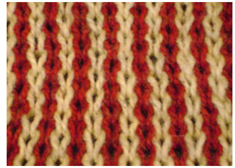
Alternating wales of red and yellow knit stitches. Each stitch in a wale is suspended from the one above it.
