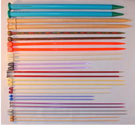
Knitting needles in a variety of sizes and materials. Different materials have varying amounts of friction, and are suitable for different yarn types.
